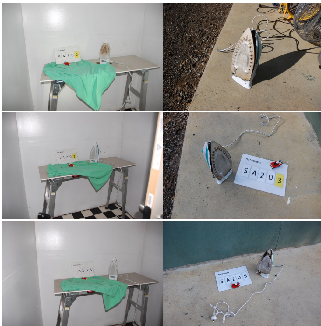
Figure 125 Before (left) and after (right) photographs of Scenario 3, Tests 1 (top), 2 (middle) and 3 (bottom).
