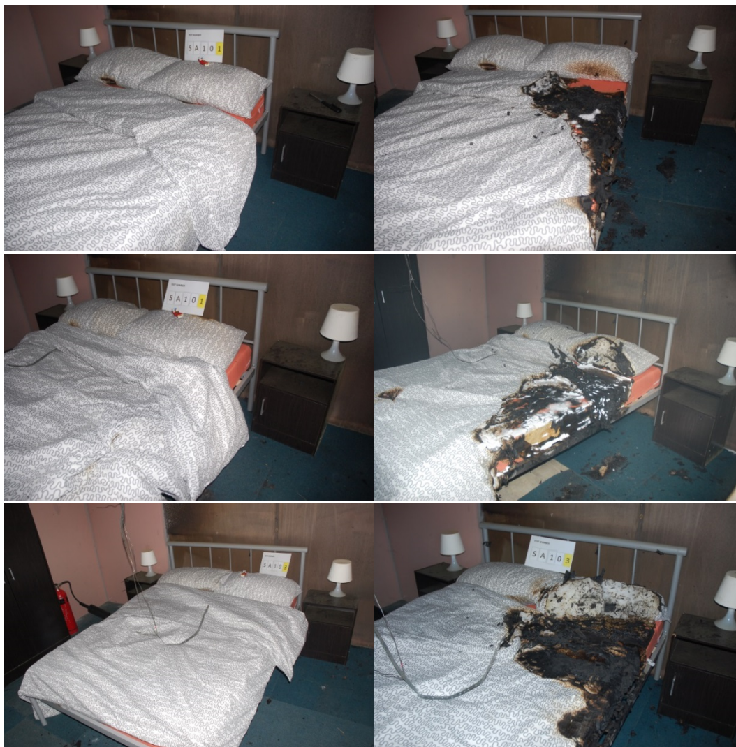
Figure 48 Before (left) and after (right) photographs of Scenario 10, Tests 1 (top), 2 (middle) and 3 (bottom).
