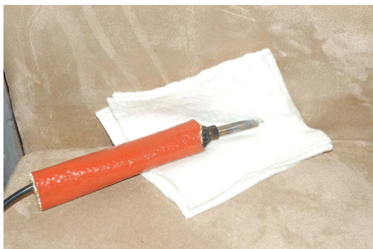
Figure 2 Soldering iron and cotton batting sheets used to initiate smouldering fires
